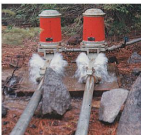
Drive Pipe - supplies the ram pump with water for a proper operation
