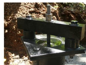
Waste Water Valve - stops the intrushing water and is mainly responsible for the over pressure
