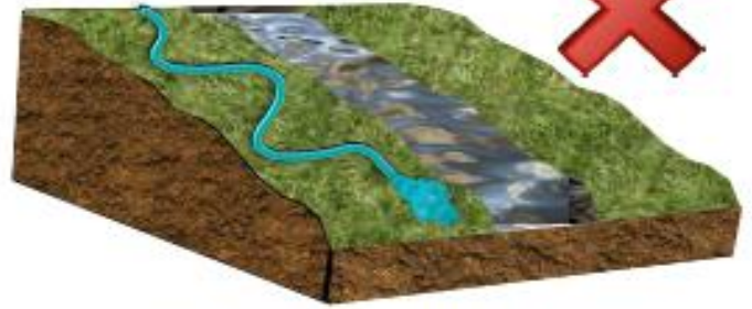
Pipework not laid straight
