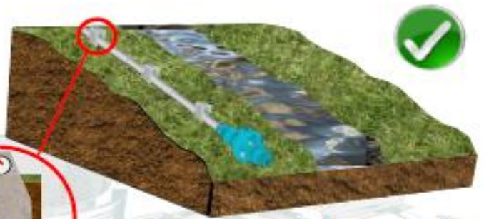
Support steel pipework when not buried
